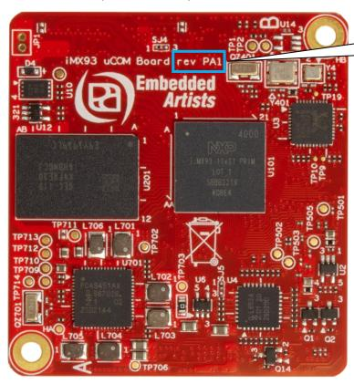
Marking on top side. The board revision (rev PA1 in this case).
