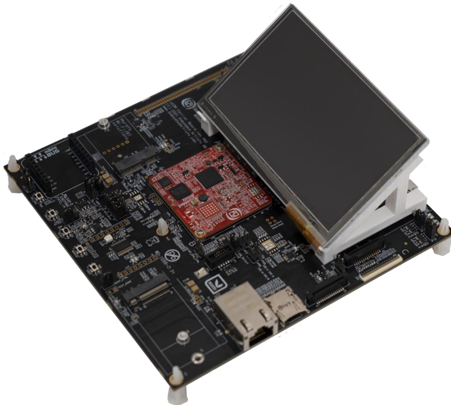
Figure 43 – LCD Mounted on uCOM Carrier Board
