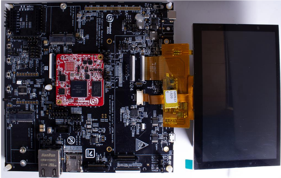
Figure 44 – 5-inch LCD Mounted on uCOM Carrier Board
