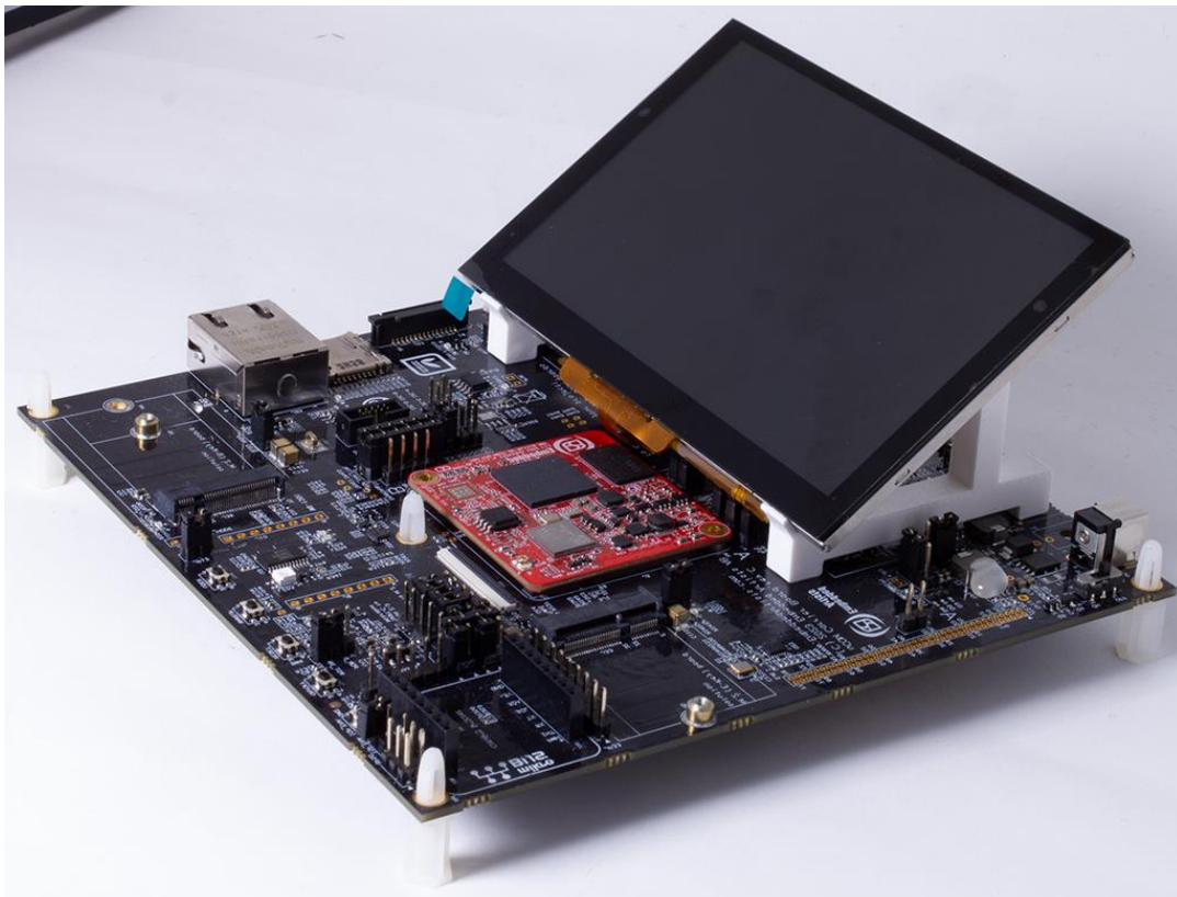
Figure 45 – 5-inch LCD Mounted on uCOM Carrier Board
