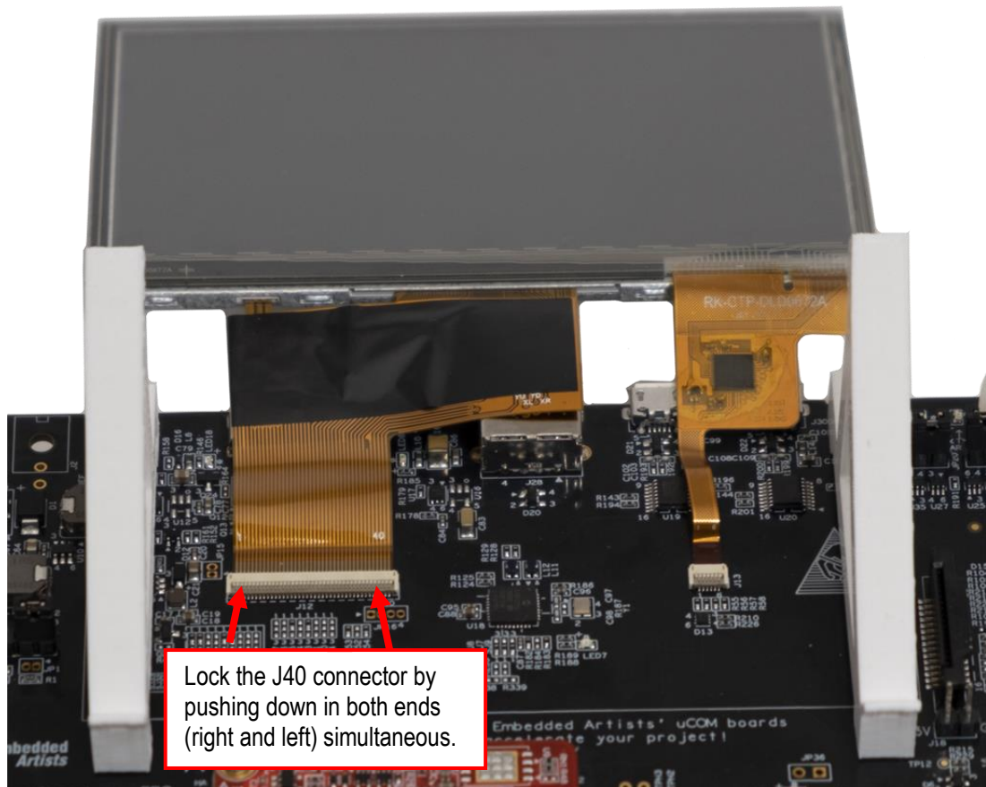
Figure 39 – Placement of LCD to Connect Flat Cables
