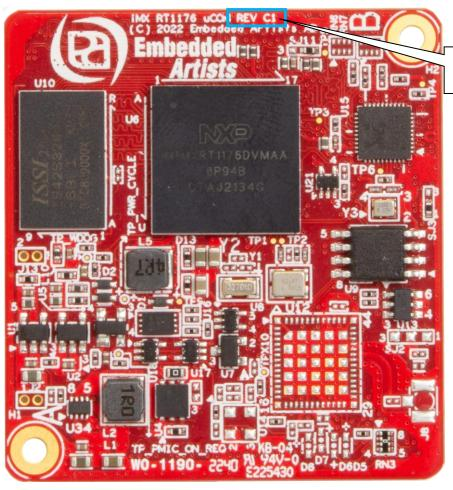
Marking on top side. The board revision (rev C1 in this
