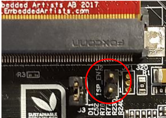
Figure 8 - J2 jumper (opened state) on a COM Carrier Board V2
