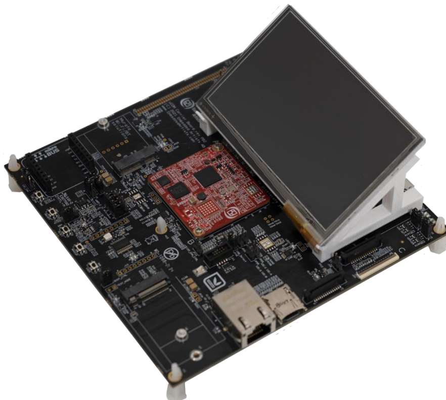
Figure 8 – LCD Mounted on uCOM Carrier Board
