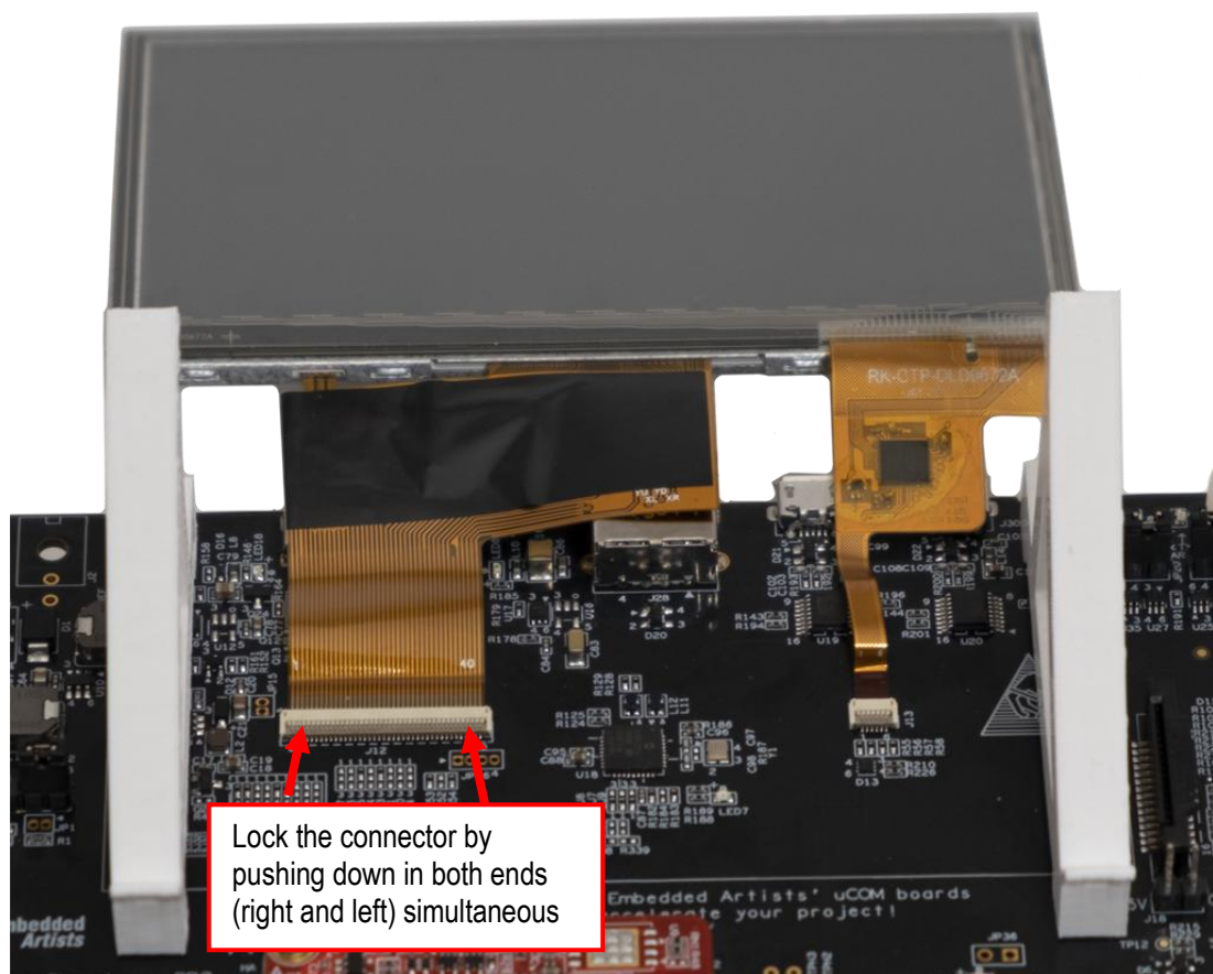
Figure 4 – Placement of LCD to Connect Flat Cables
