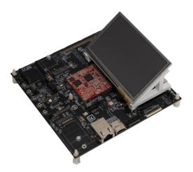
Evaluation of both display outputs are supported. For parallel RGB, the kit comes with a 4.3-inch 480x272px LCD with capacitive touch panel, and for MIPI-DSI there is a MIPI-to-HDMI bridge adapter. Software ports for several graphical frameworks exist. Users can get started with User Interface (UI) development immediately.
