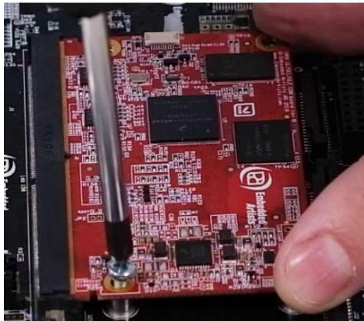
Figure 6 - Fasten board with screws
