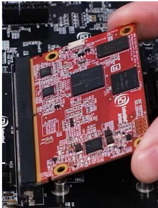
Figure 5 - COM board at an angle (Note: not fully inserted)
