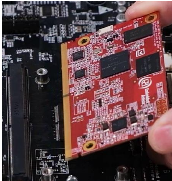
Figure 3 - Release and remove board
