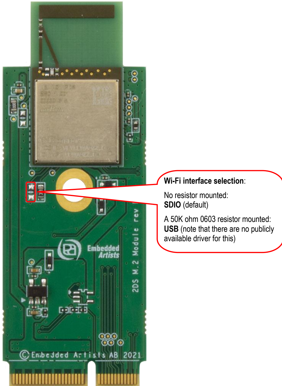
Figure 4 – 2DS M.2 Module Wi-Fi Interface Selector
