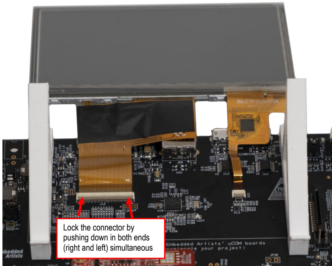
Figure 4 – Placement of LCD to Connect Flat Cables
