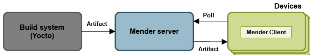
Figure 1 - Mender client/server architecture
