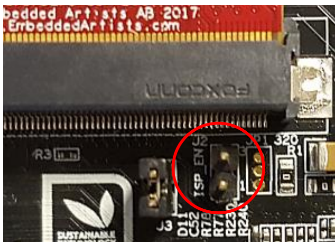
Figure 13 - J2 jumper (opened state) on a COM Carrier Board V2
