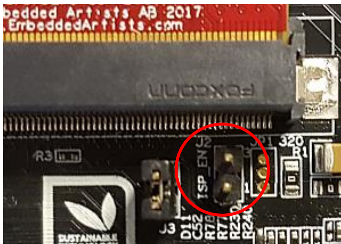
Figure 2 - J2 jumper (opened state) on a COM Carrier Board V2
