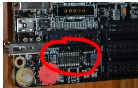
Figure 2: J10 on main board
