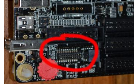
Figure 2: J10 on main board
