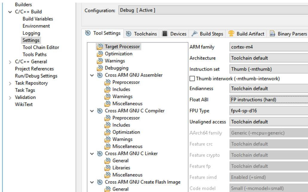
Figure 34 - Target processor
