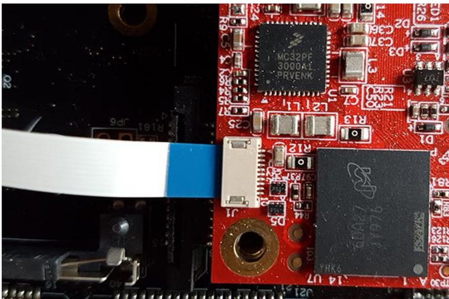
Figure 41 - Debug interface connected to COM board
