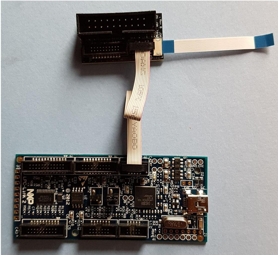
Figure 40 - LPC-Link 2 connected to Debug interface board
