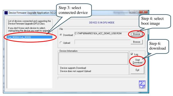
Figure 19 – Device Firmware Upgrade Application Screenshot
