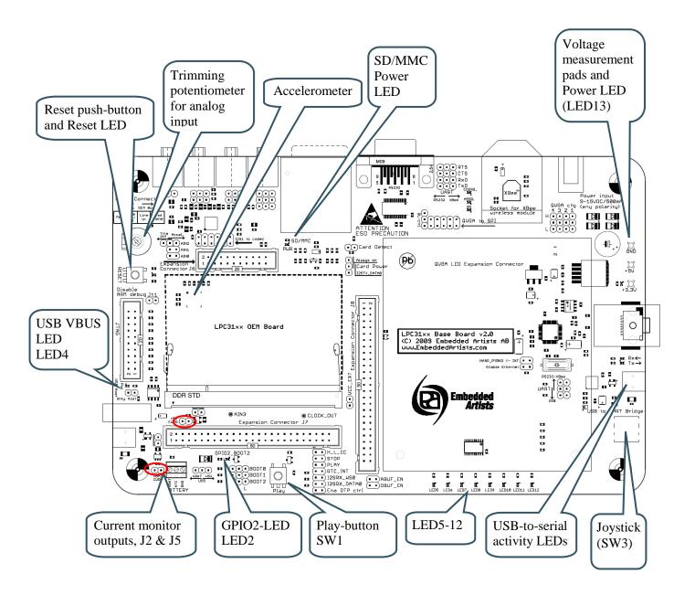
Figure 5 – LPC31xx Base Board Important Components
