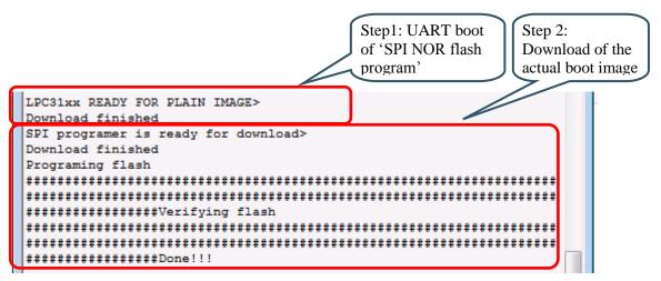
Figure 18 - Terminal Output for SPI Boot
