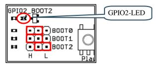
Figure 21 - GPIO2-LED Position
