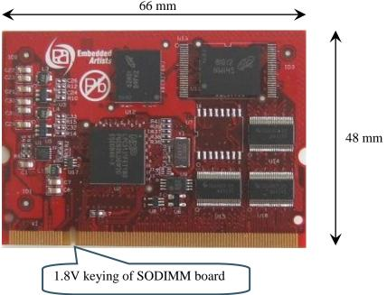
Figure 1 – LPC3131/41 OEM Board Mechanical Dimensions
