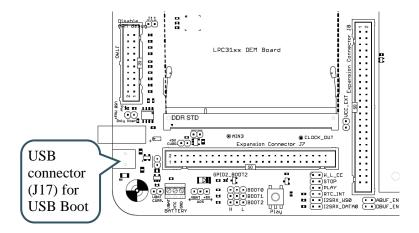
Figure 20 - LPC31xx Base Board USB Connector to LPC3131/41
