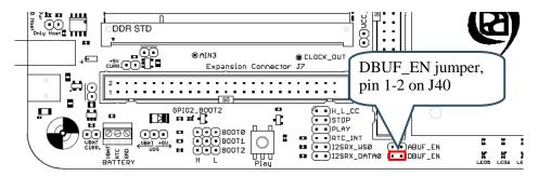
Figure 7 - DBUF\_EN jumper location on LPC31xx Base Board
