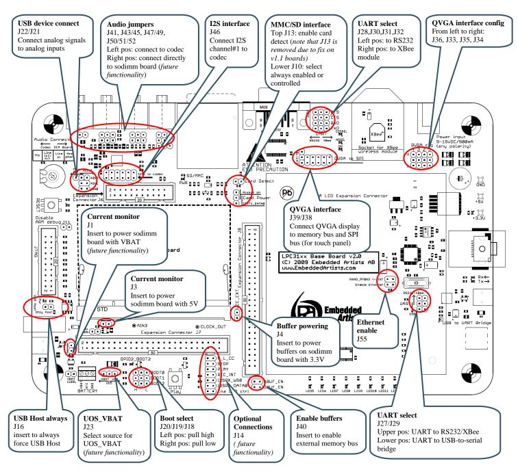
Figure 2 - LPC31xx Base Board Jumper Positions
