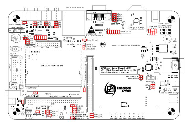
Figure 3 – LPC31xx Base Board Default Jumper Positions
