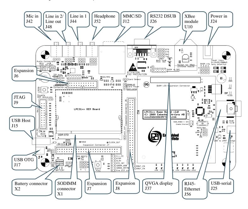
Figure 4 – LPC31xx Base Board External Connectors
