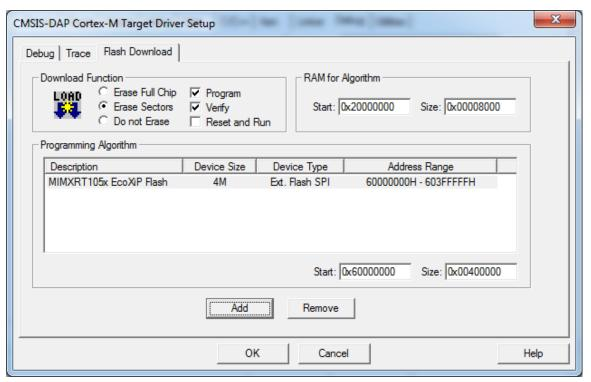
Figure 3 - Keil uVision/MDK Flash Algorithm Settings
