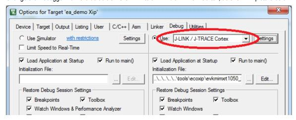
Figure 5 – Setting Debug Interface in Keil uVision
