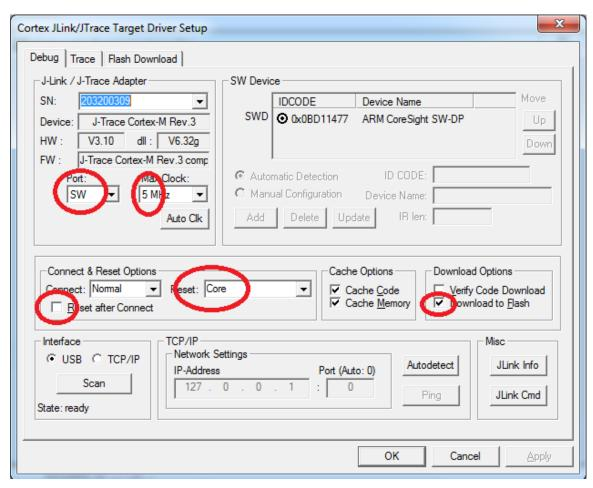
Figure 6 - Configuring J-TRACE/J-LINK Interface in Keil uVision
