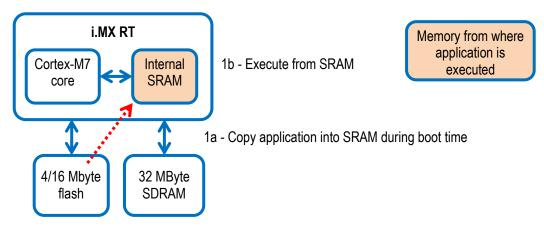
Figure 14 - i.MX RT and External Memories - Executing from SRAM
