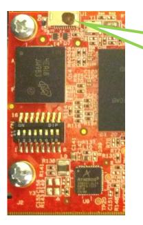
A black dot on the debug connector indicates that the board has already been reworked and is NOT affected by this note.
