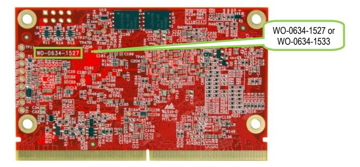
Boards marked with "WO-0634-1527" and "WO-0634-1533" are affected. These are boards called "iMX6SoloX COM board rev A". This text is also printed on the top side of the board. Boards that do not have this exact marking are not affected.
