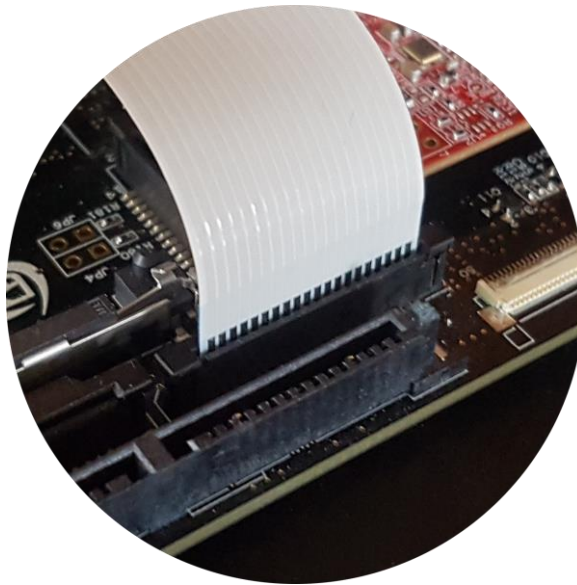
Figure 7 - Cable inserted into J21 (back)
