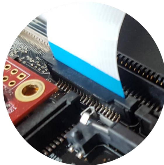
Figure 8 - Cable inserted into J20 (front)
