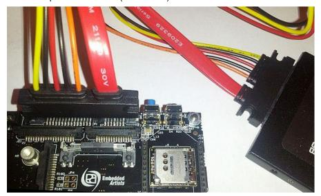
For COM Carrier Board V2 the SATA disk interface is on the M.2 connector:
