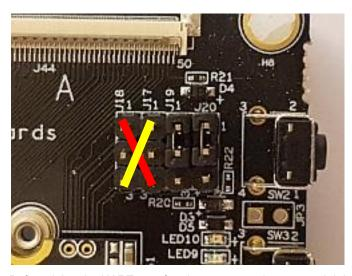
Before doing the UART test, four jumpers must be removed. It is the top four positions for J36 as shown in the figure below. When the jumpers are inserted the UART interfaces will be used by the Bluetooth interface on the M.2 connector.
