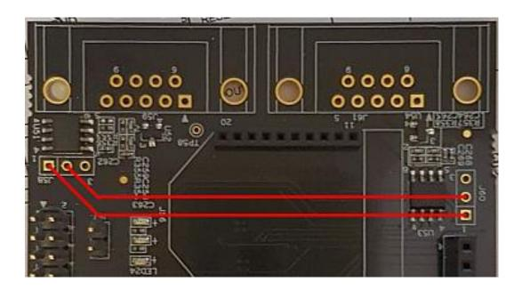
Note that for iMX6 UltraLite CAN bus 2 has been disabled in the device tree file as it conflicts with one of the UARTs. Without modifying the device tree there is no way to run the CAN tests.
