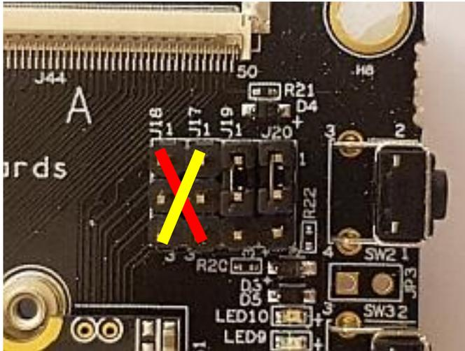
Before doing the UART test, four jumpers must be removed. It is the top four positions for J36 as shown in the figure below. When the jumpers are inserted the UART interfaces will be used by the Bluetooth interface on the M.2 connector.
