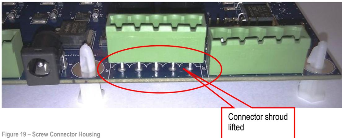
Figure 19 – Screw Connector Housing
