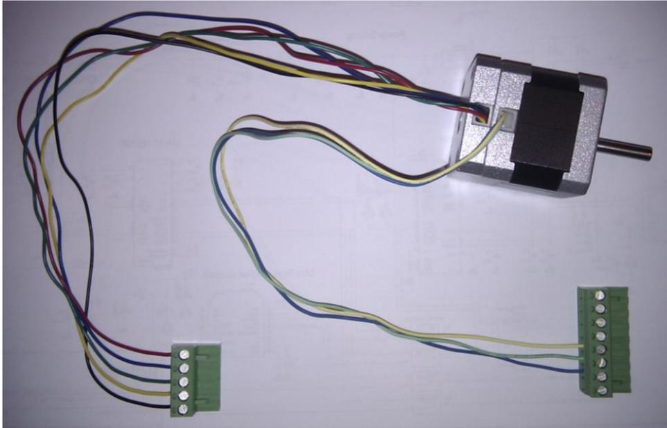
Figure 7 – BLDC motor with screw connectors
