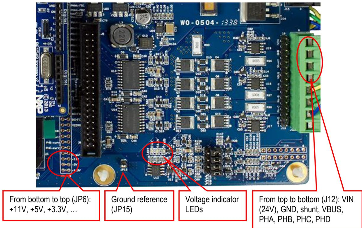
Figure 20 – Measurement Pad Locations, rev A board
