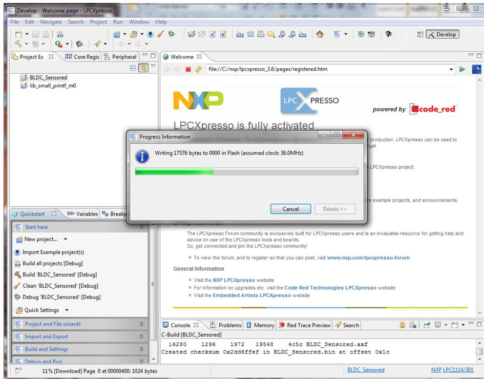
Figure 14 – LPCXpresso IDE Program Flashing in Progress
