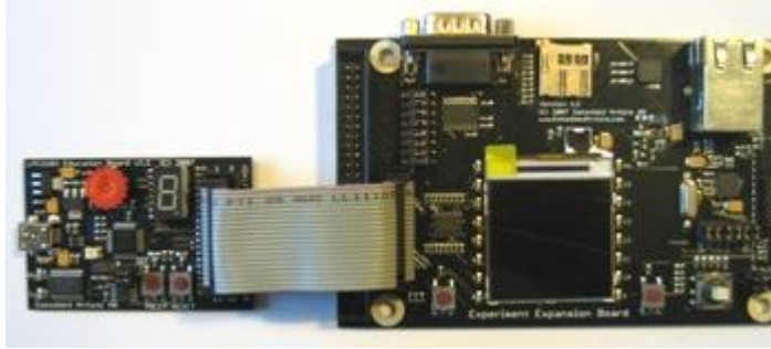
Figure 5 - LPC2103 Education Board with Experiment Expansion Board
