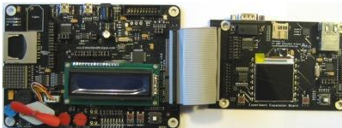
Figure 7 - LPC2148 Education Board with Experiment Expansion Board
